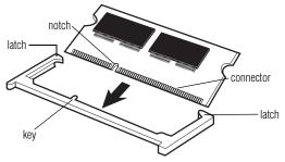
(Sample Illustration) Aligning the memory module with the socket
